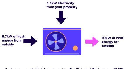
Heat energy out ÷ electrical energy in = Coefficient of Performance (COP)
